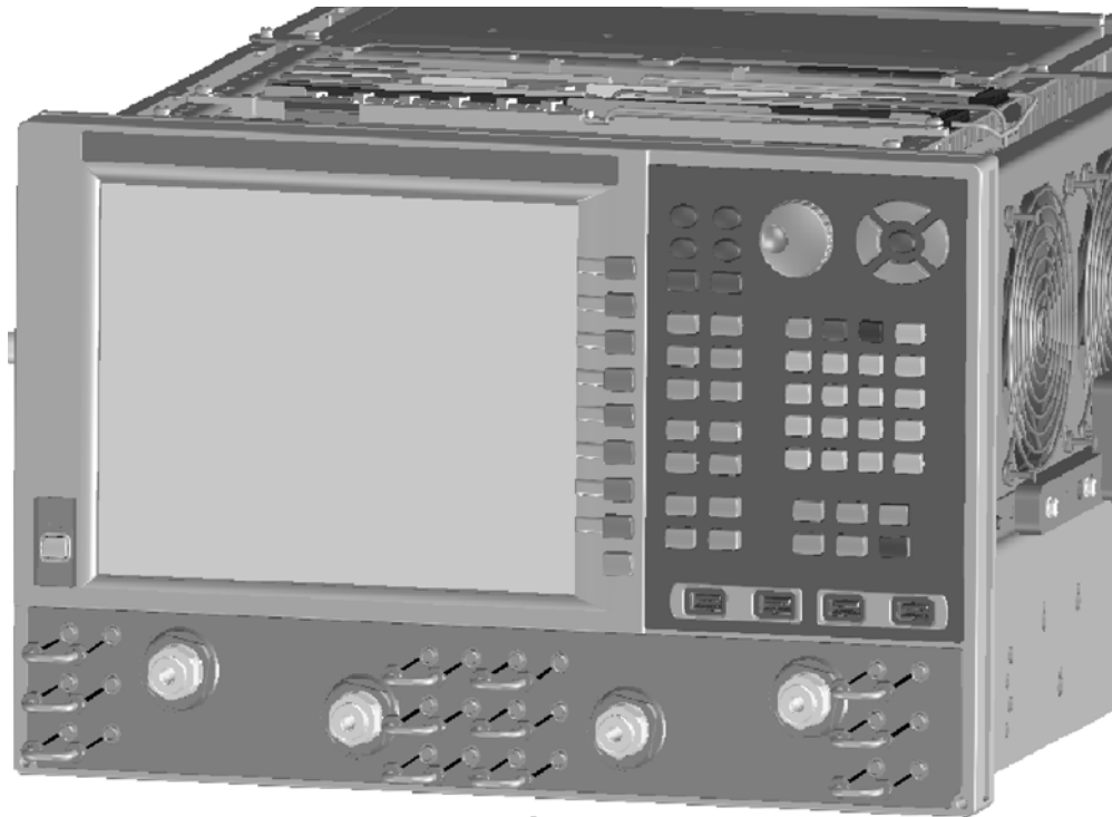
Figure 5 Front Panel Jumper Cables Installation
